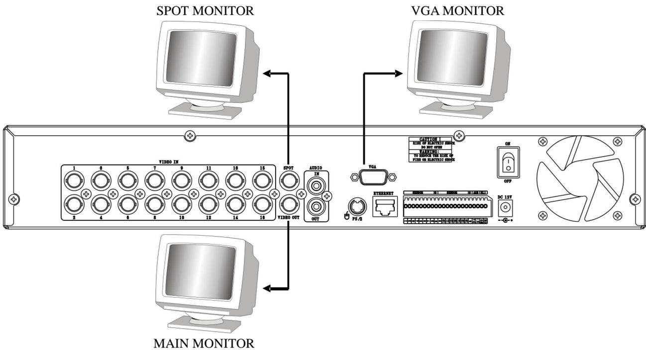
DVR supports two types of monitor output, one is Composite output (BNC connector); the other one is VGA output (DSUB-15). But you can just select one monitor output type at a time.
