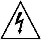
This symbol is intended to alert the user to the presence of unprotected “Dangerous voltage” within the product’s enclosure that may be strong enough to cause a risk of electric shock.
